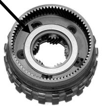
Install Front Sun Gear step facing down
