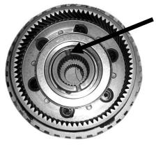
Install Rear Sun Gear with slots facing up
