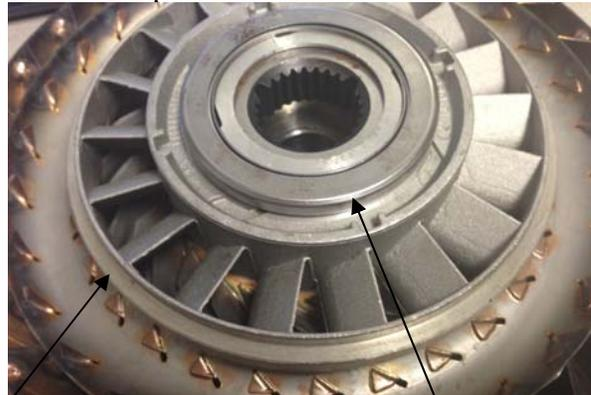
Stator placed on top of larger bearing and smaller diameter thick bearing placed on top of stator (this side up)
