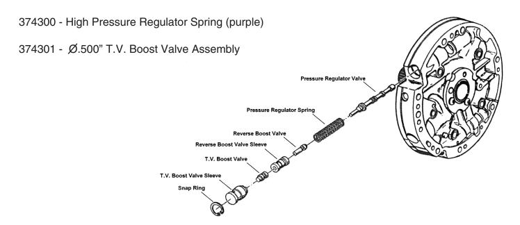
The pressure regulator assembly can be accessed by removing the pan and filter. Pump removal is not necessary. The assembly is the same on both the 200-R4 & 700-R4 transmissions.
