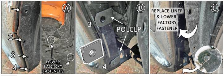
**FIGURE D** Position BMF74-FRT bracket onto mud flap points 3 and 4 then place flap, logo-side facing rear of vehicle, against liner points 3 and 4.
