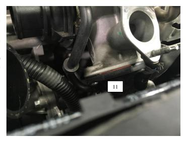
12. Reinstall OEM pipework and reattach quick connect fittings. Secure vacuum hoses appropriately in the engine bay using supplied cable ties and ensure no kinks are present.
