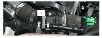
Attach the remaining length of 5mm hose to the outlet fitting on the tee piece and route the hose towards the BOV mounted on the compressor cover.
