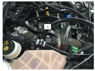
10. Undo 3 bolts attaching the BOV to the compressor cover with a T25 torx driver.
