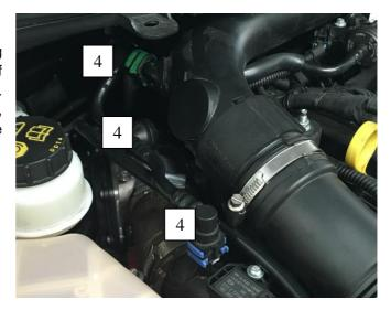
5. Ensure the coloured tabs are completely lifted prior to removal of the lines or they will not move.
