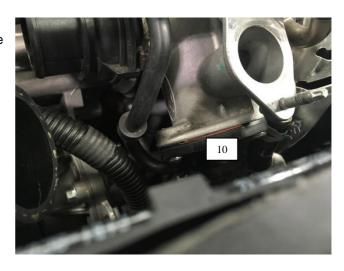
11. Install your new Turbosmart BOV in the factory location. Please note that the BOV can only be fitted in one orientation. NOTE: Ensure that the BOV flange has both Orings in place prior to installation. Use the supplied M5 bolts to secure BOV. **Torque to 6 Nm (4.23 ft.lbs).** Install hose onto BOV fitting
