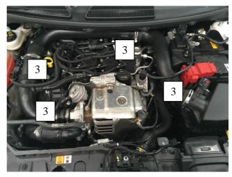
4. Unclip the emissions hardline circuit by lifting the coloured tabs and removing slightly out of the engine bay to allow for ease of assembly. There are multiple fittings in this area, including one under the turbocharger inlet pipe which is connected to the intake manifold.
