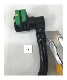
8. Cut 150mm of 5mm Vacuum hose and attach to the PCV fitting. Cut the hose now fitted on the PCV fitting to allow the 6mm tee piece to be as close to the PCV unit as possible, install associated clamps and the remaining 5mm hose onto the outlet of the tee piece which then is attached to the 90 degree quick connect fitting. Utilise a small amount of lubricant to assist.
