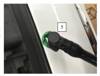
6. Identify this section of the emissions circuit hard-line, there is a 90 degree quick connect fitting with a PCV unit shortly downstream. This quick connect fitting is found directly attached to the intake manifold. This is where the signal for the BOV will be sourced from. Note: This is why it is required to "pull" the emissions line out of the bay slightly to aid in this modification.
