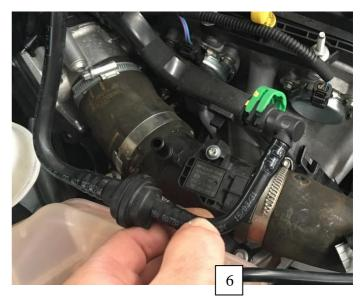
7. Cut the OEM hardline tubing off the quick connect fitting by slicing down the tube in various positions and the fitting should fall out. Take care not to cause personal injury. Repeat for the PCV end of this line.
