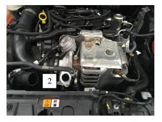
3. Remove turbocharger inlet suction pipe from air filter by undoing the hose clamps and securing nuts.
