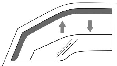
9. Raise the window until it touches the deflector. Carefully pulling the deflector outwards, roll up the window with abrupt movements. Repeat this action 4-5 times, then leave the window closed.
