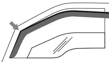
4. Shift the deflector forward, fitting the deflector frame into the channel completely. Make sure the deflector is placed above the lower window frame.
