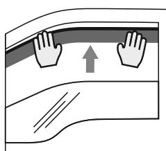
6. Starting with the front part of the deflector, insert it into the window channel.
