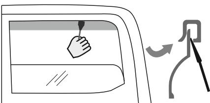
5. To ensure better installation of the deflector and better adhesion between the tape and the surface of the rubber seal, it is strongly recommended that you use the plastic blade, moving it slowly between the window's inner rubber seal and the deflector.
