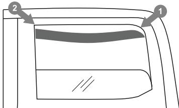
3. The deflector must be installed starting at the back. To do so, place the back part of the deflector frame into the channel and move the front part upwards. Position the entire deflector frame into the window channel, placing the frame between the fastening brackets and the rubber seal as is shown in the picture.
