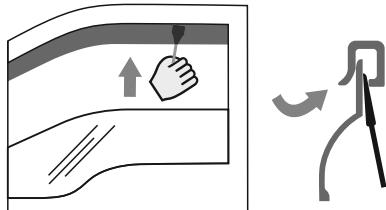
8. To ensure better installation of the deflector and better adhesion between the tape and the surface of the rubber seal, it is strongly recommended that you use the plastic blade, moving it slowly between the window's inner rubber seal and the deflector.
