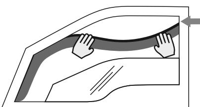
5. Bending the center part of the deflector outwards, insert the back part of the deflector into the channel, leaving a gap above it.
