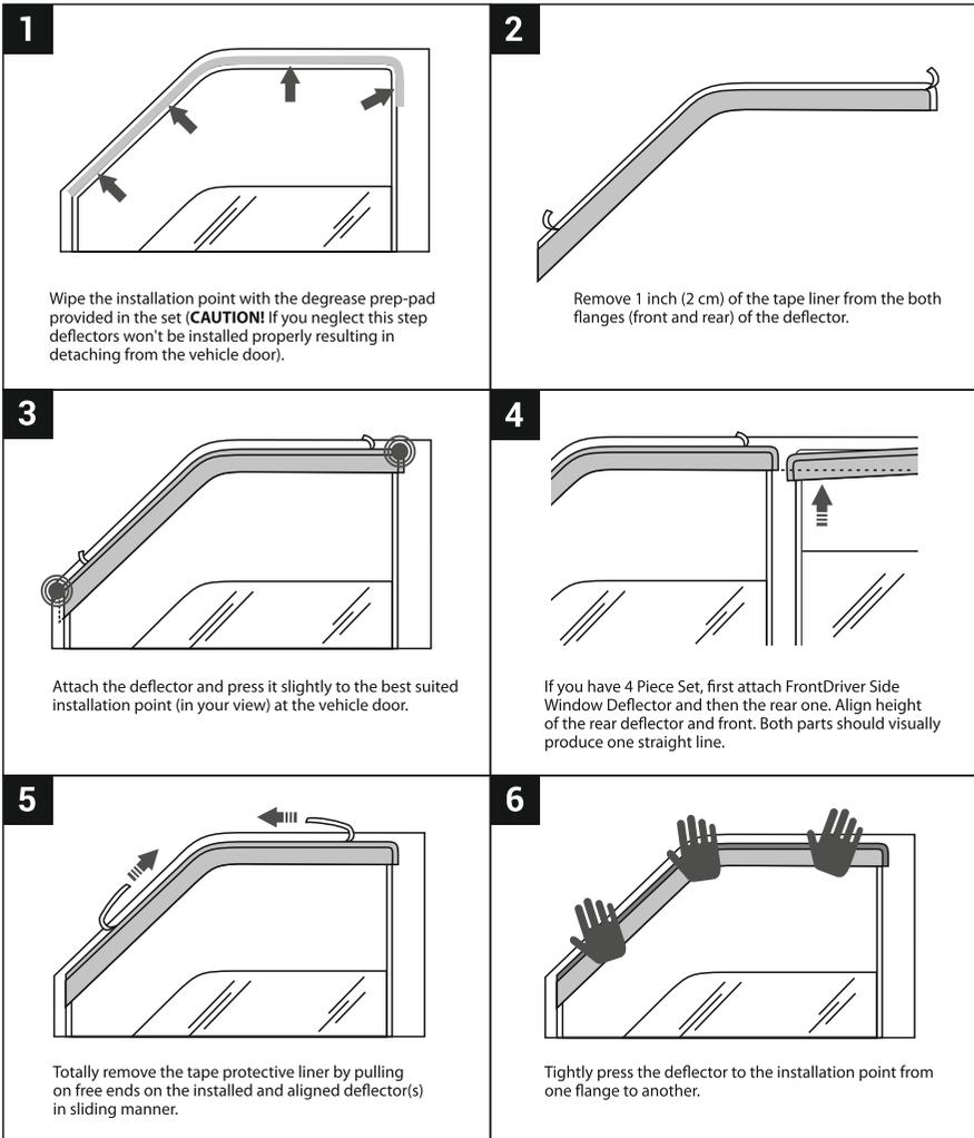
Wipe the installation point with the degrease prep-pad provided in the set (**CAUTION!** If you neglect this step deflectors won't be installed properly resulting in detaching from the vehicle door).
