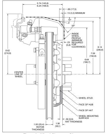
Figure 2. Wheel Clearance Diagram
