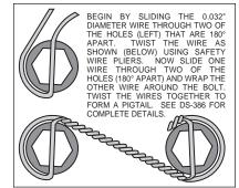
Figure 3. Safety Wire Diagram
