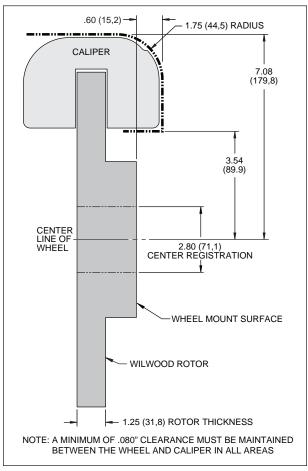
Figure 2. Wheel Clearance Diagram
