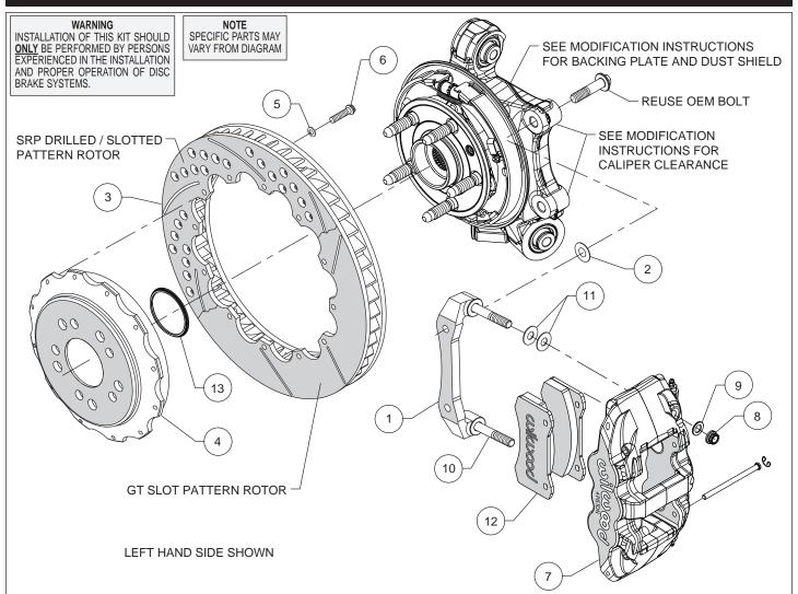
Figure 1. Typical Installation Configuration
