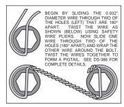
Figure 4. Safety Wire Diagram
