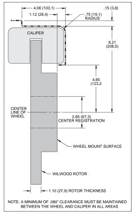
Figure 2. Wheel Clearance Diagram
