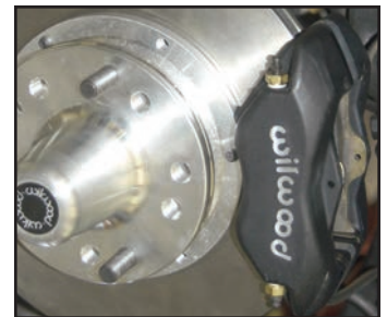
Photo 11 Caliper Bleeding Position
