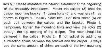
bolts. **NOTE:** The end of each bolt must be flush with or slightly protruding from the head of the clinch nut, as shown in Figure 3. If necessary place spare shims between washer (4) and caliper mounting ear to achieve the proper clinch nut engagement. Once the caliper alignment and clinch nut engagement are correct, remove the bolts one at a time, apply red *Loctite*® 271 to bolt threads, and torque to 40 ft-lb.
