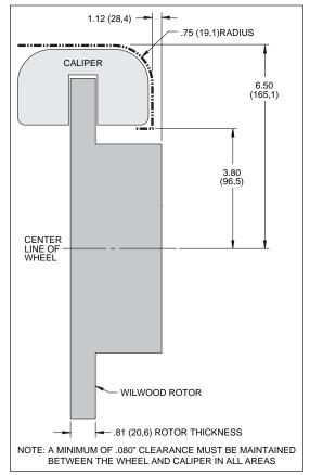
Figure 2. Wheel Clearance Diagram
