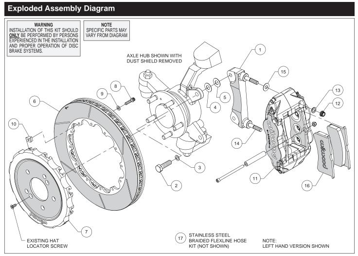
Figure 1. Typical Installation Configuration
