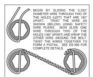
Figure 3. Safety Wire Diagram
