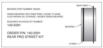
Figure 2. Loose Fit Flange Bearing Configuration
