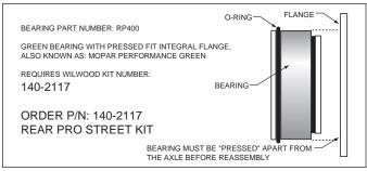
Figure 1. Press Fit Flange Bearing Configuration
