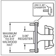
Figure 5. Axle Flange Maximum Dimension
