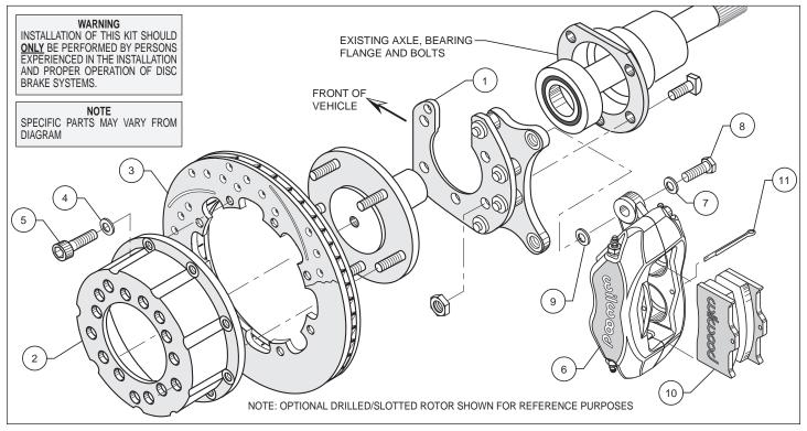
Figure 3. Typical Installation Configuration
