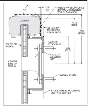
Figure 4. Wheel Clearance Diagram
