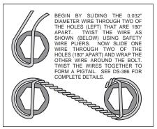
Figure 3. Safety Wire Diagram
