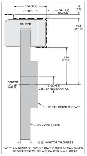
Figure 2. Wheel Clearance Diagram
