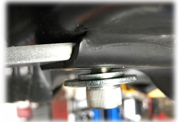
Figure 1: Correct order of install for bolt and washers
