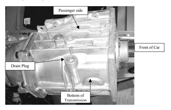
For TR3650 vehicles the drain plug is directly on the bottom of the transmission pointing at the ground. (555-7363)
