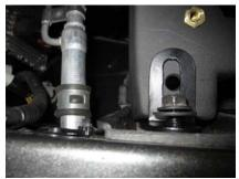
14. Attach the small L bracket to the mounting tray using the factory bolt. Than attach the bracket to the box using the provided hardware.
