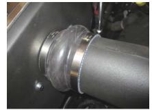
17. Press the Volant duct into the hump hose and sleeve and tighten the remaining clamps.
