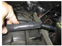
8. Re-install the factory elbow and attach the  $\frac{3}{4}$  in breather hose.
