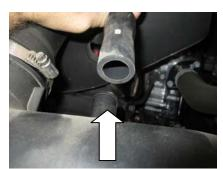
3. Remove the breather hose from the air box by pulling straight out.
