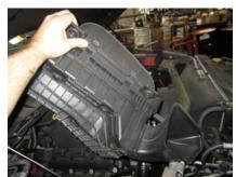
4. Remove the factory air box by pulling up and over the grommet posts.
