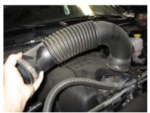
2. Loosen the clamps holding the duct to the throttle body and air box than remove the air duct.
