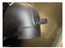
16. Press the ATS sensor into the½ rubber grommet.
