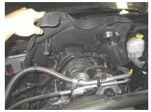
5. Remove the engine cover by pulling up and forward.
