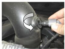
1. Disconnect the negative battery cable and remove the ATS sensor by twisting it out.
