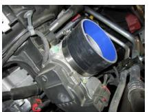
9. Attach the sleeve onto the throttle body with the #56 clamp.
