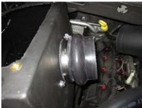
15. Attach the hump hose to the volant box using the #64 clamp.
