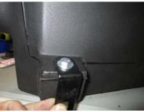
11. Attach the large L bracket to the headlamp side of the volant box using the provided hardware.
