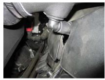
18. Attach the breather hose to the Volant  $\frac{3}{4}$  in elbow.
