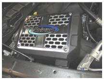
21. Attach the Volant filter box lid and re-install the negative battery cable.
