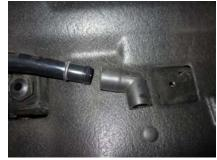
6. Remove the factory elbow from the factory breather hose.
