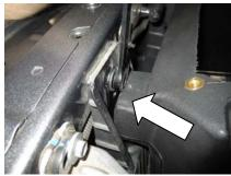
13. Attach the long L bracket to the tray using the factory bolt.
