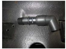
7. Attach the ¾ in straight fitting into the factory elbow.
