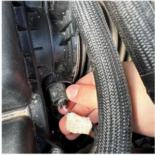
1. Disconnect the electrical connection on the air temperature sensor by pressing on the tab and pulling.
