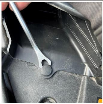
5. Use a trim removal tool or similar to remove the clip at the front of the air scoop.
