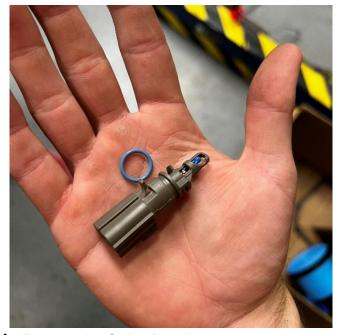
4. Remove the O-ring from the temperature sensor.
