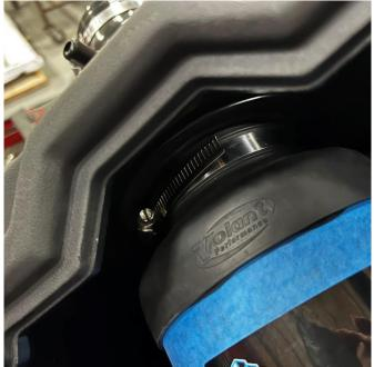
8. Tighten the clamp to secure the filter to the air duct using an 8mm socket and ratchet.
