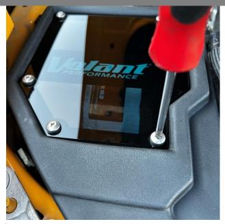
14.Place the Volant lid on top of the airbox and tighten to the air box using the lid screws and a Phillips screwdriver.
