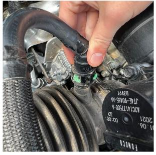
2. Remove the PCV line by pressing the green tabs on the fitting up and out then pulling the fitting off.
