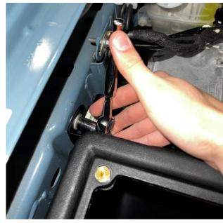
12. Align the supplied bracket to the threaded hole in the frame and use a 10mm socket and the stock bolt from removal step 3 to secure the Volant airbox to the vehicle.
