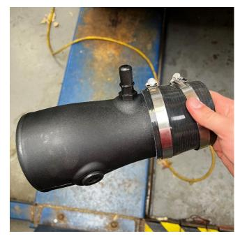
3. Install the silicone reducer to the smaller end of the Volant air duct. Prep the Ø3.5" and Ø3.25" clamps for install by sliding them over the silicone reducer. Use an 8mm socket and ratchet to tighten the Ø3.5" clamp over the duct. Leave the Ø3.25" clamp loose for installation.
