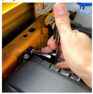
3. Use a 10mm socket and rachet to remove the bolt located behind the stock air box. Save bolt for installation step 12.
