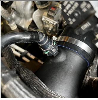
10. Carefully install Volant air intake and fit the silicone reducer over the stock turbo inlet pipe. Tighten Ø3.25" clamp reconnect the PCV line to the Volant air duct by pressing it over the fitting until it clicks into place.
