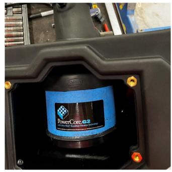
7. Install the air filter (61509 Powercore Filter shown) and air filter clamp directly over the end of the air duct inside the air box. Fit pre-filter over filter if desired.
