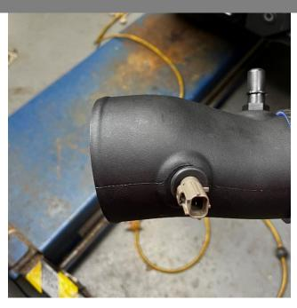
5. Install the temperature sensor to the air duct by fitting it through the rubber grommet. Make sure sensor is oriented as shown.
