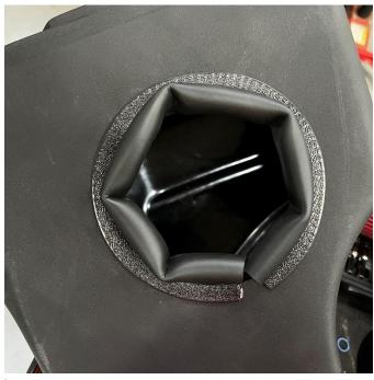
1. Install filter bulb seal trim onto the Volant air box.
