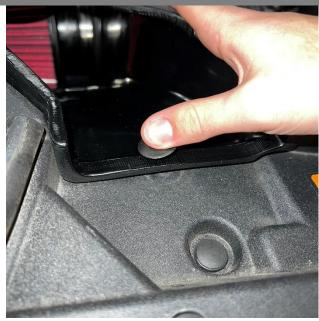
13. Use the supplied Christmas Tree clip to secure the scoop portion of the Volant airbox to the stock air intake tray.
