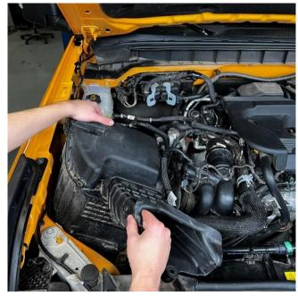
7. Carefully remove the stock air intake by pulling up and out.
