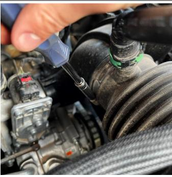
Loosen the clamp securing the air duct to stock turbo inlet pipe and pull the duct off the inlet pipe.
