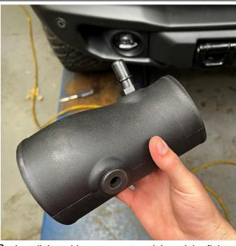
2. Install the rubber grommet and thread the fitting onto the Volant air duct.
