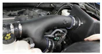
16. Adjust air duct as necessary and tighten all clamps using a ratchet and 8mm socket or flat head screw driver. **NOTE:** Make sure to tighten the filter clamp as well.
