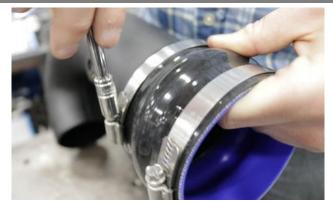
12. Install the hump hose onto the Volant air duct along with two #64 clamps and tighten using a ratchet and 8mm socket or flat head screwdriver. Leave clamp on open end of hump hose loose.
