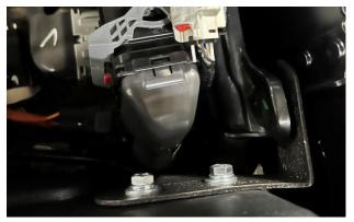
6. Insert push clip on factory wiring harness mount into hole on bracket
