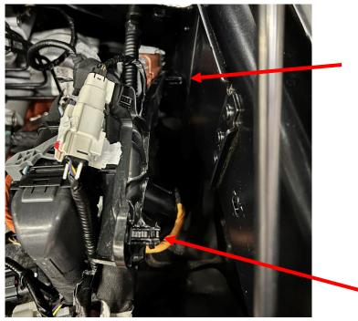
11. Using a trim removal tool, carefully pull the plastic wiring harness mount from the inner fender.
