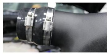
14. Insert larger end of reducer onto Volant air duct using #56 clamp. Place #48 clamp on the smaller side. Tighten #56 clamp only using a ratchet and 8mm socket or flat head screwdriver.
