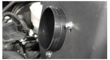
Locate three 6mm x 16mm bolts, three .25" x .63" flat washers, and three .25" lock washers. Attach filter adapter to air box and tighten using a ratchet and 10mm socket.
