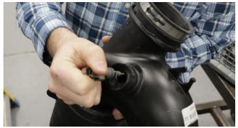
9. Remove the air temp sensor from factory duct. Save for Install Step 17.
