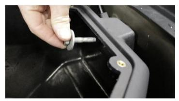
5. Attach the Volant air box to the fender with the bolt from **Removal Step 4** using a ratchet and 13mm socket.
