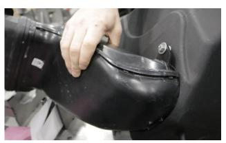
3. Install factory scoop to Volant air box using provided 6mm-25 bolt with flat washers, lock washer, spacer, and nut using 10mm socket or wrench.
