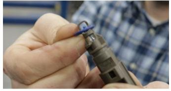
10. Remove O-ring from the temp sensor.
