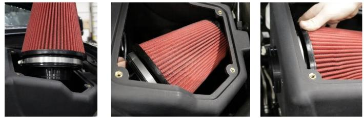
9. Insert the filter into the air box with the adapter side down. Rotate the top of the filter down into the air box and rotate the filter around and push the adapter through air box.
