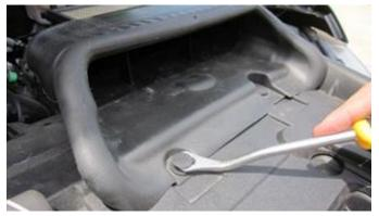
6. Remove the two plastic clips from the factory air scoop. Save clips for Install Step 7.
