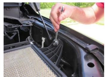
4. Use a ratchet and 13mm socket or wrench to remove the bolt holding the air box to the vehicle. Save bolt for Install Step 5.
