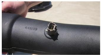
11. Locate air temperature sensor from removal step 9 and Volant air duct. Install sensor into grommet with tab facing the closest end of air duct.
