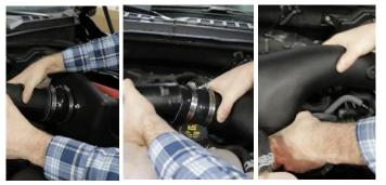
15. Install Volant air duct into vehicle by placing the hump hose onto the filter adapter. Then place reducer onto the upper stock inlet. Rotate duct down and into the straight sleeve.
