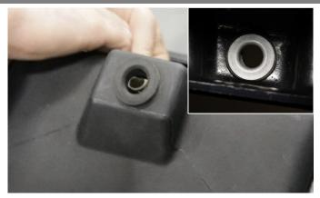
Insert the factory grommet from Removal Step
