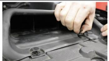
7. Reinstall factory scoop and attach with clips from **Removal Step 6**.
