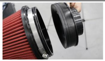
8. Place the filter clamp on the filter and insert the filter adapter as shown. Do not tighten clamp.
