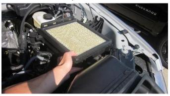
Remove the bottom box assembly by pulling it up and out. Remove the rubber grommet and metal bushing from factory air box. Save for Install Step 4.
