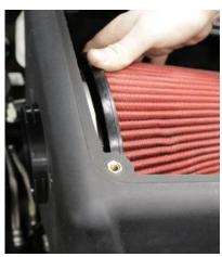
**10.** Insert the filter into the air box with the adapter side down. Rotate the top of the filter down into the air box and rotate the filter around and push the adapter through air box.
