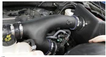
17. Adjust air duct as necessary and tighten all clamps using a ratchet and 8mm socket or flat head screw driver. NOTE: Make sure to tighten the filter clamp as well.
