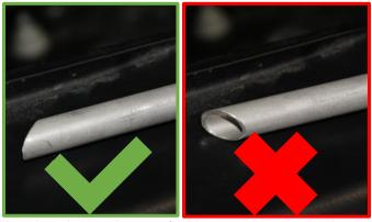
Use the above pictures for the correct way to place the vent line fitting for **Install Step 2**.
