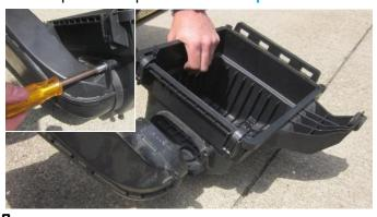
**8.** Remove the bolt attaching the scoop to factory air box using an 8mm socket. Remove the factory air scoop from the bottom of the air box.
