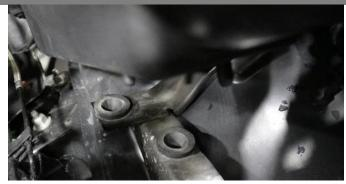
**6.** Install Volant air box into the vehicle by inserting stems on bottom of Volant air box into factory grommets.
