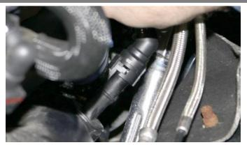
1. Unclip the quick disconnect vent hose.
