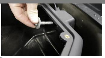
Attach the Volant air box to the fender with the bolt from Removal Step 4 using a ratchet and 13mm socket.
