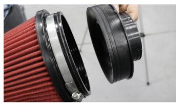
**9.** Place the filter clamp on the filter and insert the filter adapter as shown. Do not tighten clamp yet.
