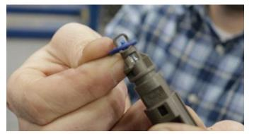
${\bf 10.}$  Remove O-ring from the temp sensor.
