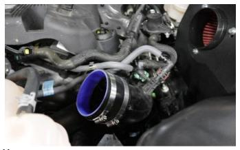
**14.** Install the straight sleeve onto lower factory inlet with #64 clamp. Tighten clamp using a ratchet and 8mm socket or flat head screwdriver. Leave clamp on open end of straight sleeve loose.
