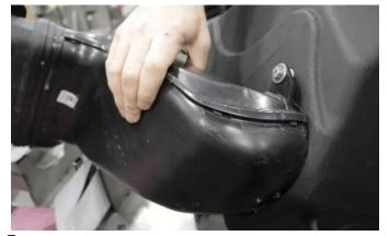
Install factory scoop to Volant air box using provided 6mm-25 bolt with flat washers, lock washer, spacer, and nut using 10mm socket or wrench.
