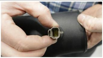
**12.** Install air temp sensor from **Removal Step 9** with the tab facing the short end of the duct, as shown.
