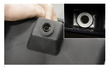
4. Insert the factory grommet from Removal Step 7, then install the metal bushing into grommet from inside box as shown.
