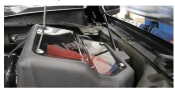
**19.** Install lid using provided 4 truss head screws with rubber washers and Philips head screwdriver.
