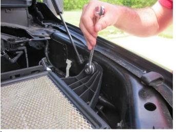
**4.** Use a ratchet and 13mm socket or wrench to remove the bolt holding the air box to the vehicle. Save bolt for **Install Step 7**.
