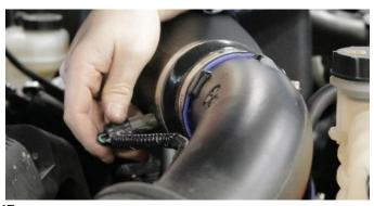
**18.** Clip wiring harness on air temperature sensor.
