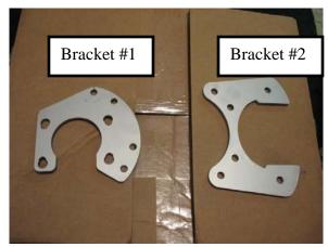
Take bracket #1 (shown below) and align it with the T-bolts you just installed. The curved part of the bracket #1 can point towards the front or rear of the car. This will determine if you caliper is going to be front mounted or rear mounted. As a general rule of thumb, you mount the caliper on the opposite side of the axle than the shock is on. Caliper clearance is the issue here. If your caliper will clear the shock it is ok to mount
