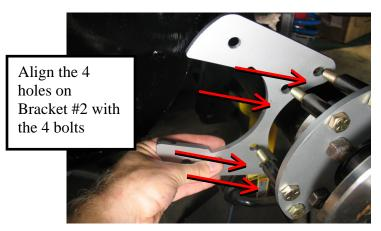
Take four of the eight nuts and lock washers and tighten down bracket #2 to bracket #1.
