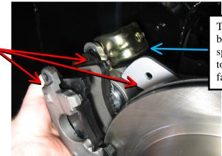
The zinc plated bracket with spring attached to it needs to face upwards.
