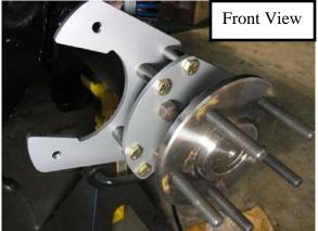
Slide the rotor onto the studs. The rotors are drilled for both Mopar / Ford and Chevy bolt patterns. Hand thread two lug nuts to seat the rotor in place for test fitting. If the center hole in the rotor that measures 2.78" is too small you will need to machine the rotor to fit. If the recess area of the rotor is too small to go over your axle hub you will need to machine the axle to fit the  $6 \ 3/16$ " rotor hat. These are the only rotors available for this kit.
