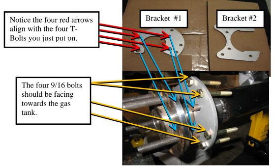
Attach the four new T-bolts and lock washers and tighten them in a star pattern using a <sup>3</sup>/<sub>4</sub>" wrench or socket. Torque the axle flange brackets to 55 ft/lb.
