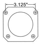
This kit is for axles with a 3 1/8" spread center to center on the top two bolt holes (pictured left). If your axle flange measures 3 3/8" from center to center, you need our kit FSCRD01 or FSCRD65. Call 800.405.2000 for further assistance.
