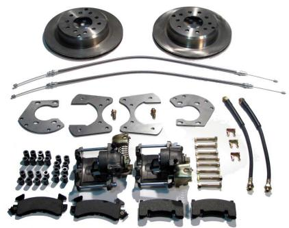
This kit is for Ford 9" rear axles with the large (3.15") style bearing, either Torino style rear ends or the old style of large bearing. This kit is designed to work with axles with either GM 5 x 4.75 Bolt Pattern and 7/16" wheel studs or Ford 5 x 4.5 Bolt Pattern and  $\frac{1}{2}$ " wheel studs. Rotor center measures 2.78".
