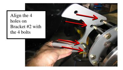
Take four of the eight nuts and lock washers and tighten down bracket #2 to bracket #1.
