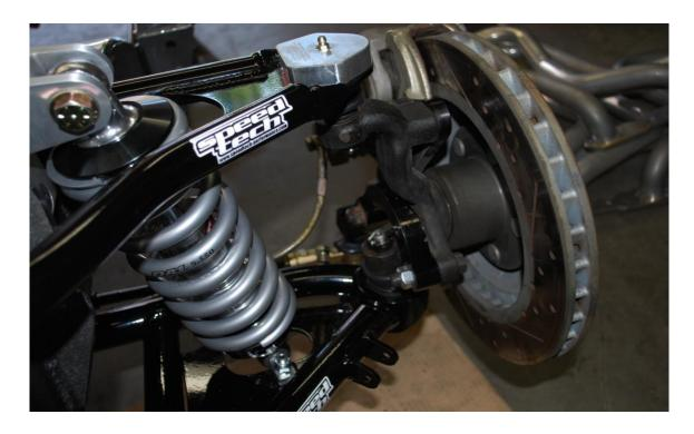
9. Factory spindles can be reinstalled. For optimum performance we recommend using ATS AFX tall spindles. Tighten the lower ball joint to 60 ft/lbs and install the cotter pin. Tighten the upper ball joint to 40 ft/lbs. and install the cotter pin.
