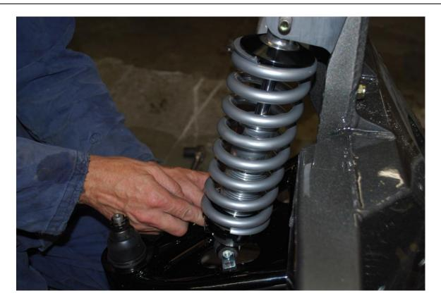
7. Install the lower side of the shock into the lower control arm. You have the option to install the T bar on either the top or the bottom of the mounting pad. Installing it on the bottom will lower the car approximately an additional  $1\frac{1}{4}$ ". Install the top shock eyelet into the frame bracket. Tighten bolts to 20 ft/lbs.
