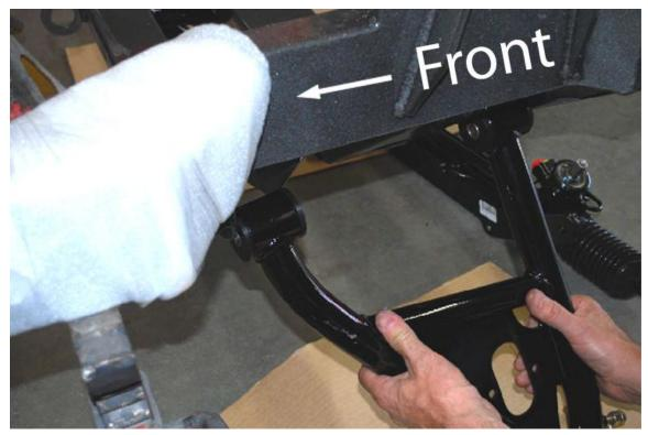
4. Install the lower control arms. Begin control arm installation by sliding the frame end up into the frame pockets, the straight tube should be located to the rear.
