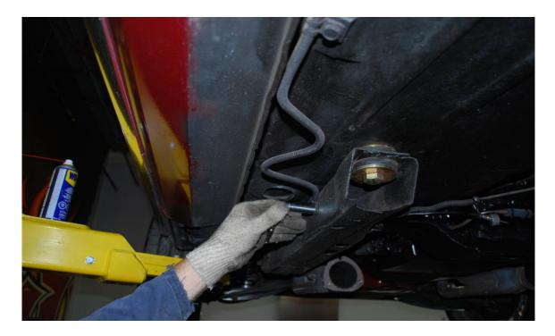
14. Once you have removed your original sub frame there are a couple of ways to proceed. If you are using a two post hoist, we recommend you install the motor and transmission into the Speedtech sub frame and then install the completed unit into the car. This allows more room to perform some detail work on the entire assembly without the car's front clip in the way.
