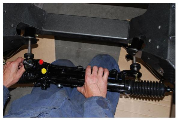
You must remove the rack from the mounting bracket to get the driver side bolt into it's position in the bracket. Apply anti-seize lubricant to the shank of the bolts, install into bracket, then reinstall bracket onto rack body.
