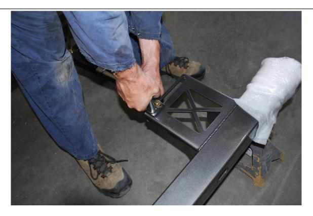
3. Install the transmission cross member. Do not fully tighten the bolts at this time to allow adjustment later when installing the engine and transmission.
