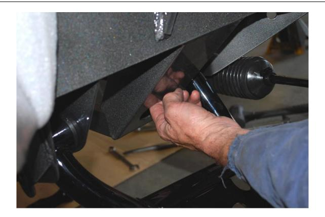
The lock nuts that are provided with the lower control arms must be installed through the hole in the bottom of the sub frame, a small amount of red Loctite is suggested. At this time you can torque all 4 lower control arm nuts to 70 ft/ lbs.
