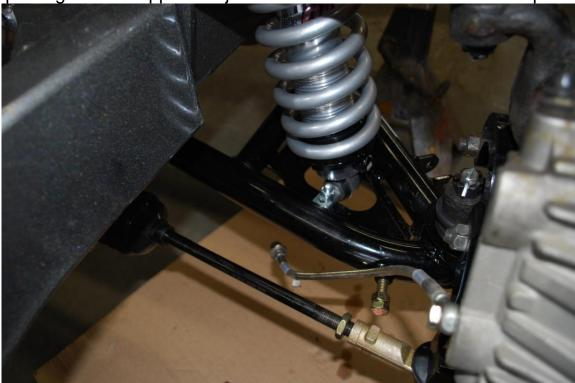
10. Install the new steering arms using either your original hardware or new grade 8 hardware. Install the outer tie rod ends into the steering arms, torque to rack and pinion manufacturer specs.
