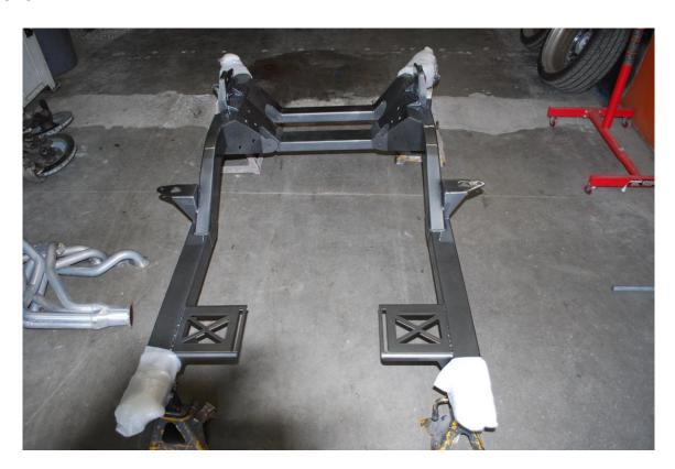
2. Install the supplied motor mounts. Do not fully tighten the bolts at this time to allow adjustment later when installing the engine.
