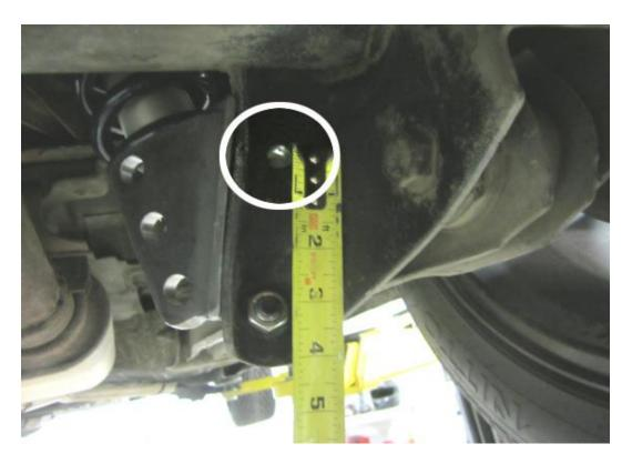
Using the pre-drilled hole in the Speedtech bracket as a guide, drill a 7/16" hole in the side of the factory bracket. Use one  $7/16 \times 11/4$ " bolt, (2) 7/16" washers, and one 7/16" Nylock Nut and tighten down.
