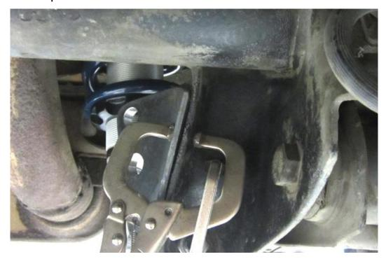
Measure and mark the rear side of the factory bracket 3" above the 1/2" bolt. Using your mark, drill a 7/16" hole through both the factory and Speedtech bracket. Install one  $7/16 \times 11/4$ ", (2) 7/16" washers, and one 7/16" Nylock nut through the hole and tighten.
