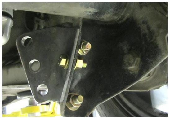
**DO NOT** skip these steps. Both of the 7/16" bolts must be installed to properly secure the coilover conversion bracket.
