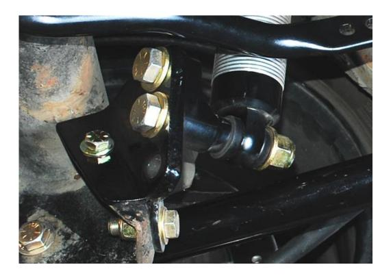
If you want additional ride height drop or lift, simply rotate the adapter accordingly to move that longer bolt to one of the other holes.
