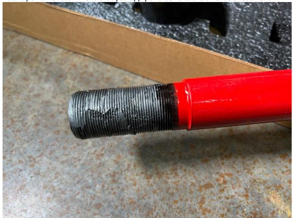
f. Note – the ends have different threads. One is standard right-hand thread and one is reverse left-hand thread, meaning you will spin in one end in clockwise and the other end will go in counterclockwise. This also means that the ends only go in one end of the adjuster. Pay attention to the tube and you will see there are bevels on each end. One of the bevels will have
