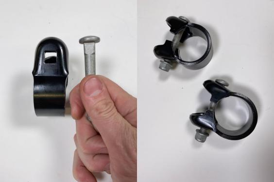
d. Slide the clamps onto the adjuster tube (preferably with the clamps nut facing the same direction), and then snug the nut up so that the clamp still rotates but does not slide off. Use your 15mm socket or wrench
