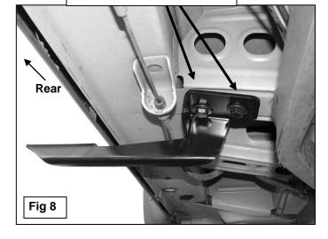
Use these (2) holes. Remove foam as necessary. Insert 10mm Bolt/8mm Nut Plate
