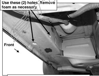
(Fig 1) Driver side front mounting location
