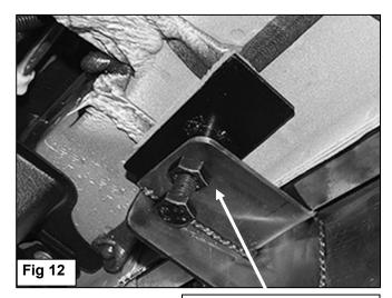
Tighten 10mm Jam Nut to lock adjustment in place
