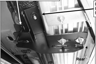
(Fig 9) Passenger rear Bracket with Running Board
