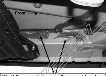
(Fig 1) Remove plastic cover. Remove rubber plugs in factory holes. NOTE: Driver side pictured
