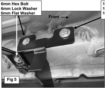
10mm Hex Bolt 10mm Lock Washer 10mm STD Flat Washer NOTE: To insert a 10mm Threaded Insert into the large factory hole, check for fit and/or use 1/2" drill bit as necessary
