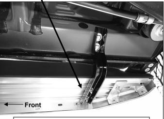
(Fig 9) Rear Bracket installation pictured
