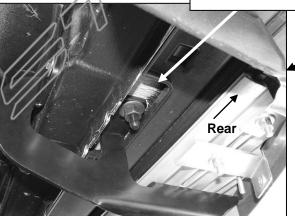
(Fig 13) Passenger side rear Bracket pictured
