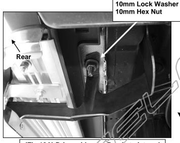
(Fig 12A) Driver side rear Bracket pictured
