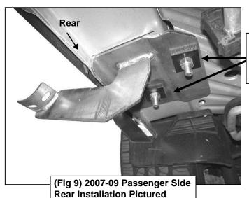
12mm x 45mm Bolt Plate 12mm Square Washer 12mm Lock Washer 12mm Hex Nut 10mm x 35mm Bolt Plate 12mm Square Washer 10mm Flat Washer 10mm Lock Washer 10mm Hex Nut
