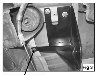
10mm x 30mm Hex Bolt 10mm Lock Washer 10mm Hex Nut 10mm Flat Washers
