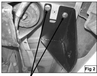
(Bolt Plate) 10mm x 30mm Hex Bolts 10mm Lock Washers 10mm Flat Washers
