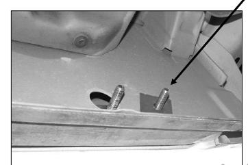
Fig 5 Super Cab passenger side rear mounting location pictured. Shown with Plastic Retainer in place
