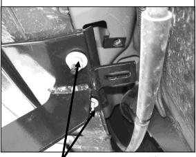
10mm x 30mm Hex Head Bolts 10mm Flat Washers 10mm Lock Washers 10mm Hex Nuts
