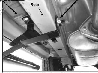
(Fig 7) Passenger Side Rear Mounting Bracket
