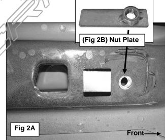
Vehicles with threaded hole in body panel use: 8mm x 35mm Hex Bolt 8mm Large Flat washer 8mm Lock Washer 6mm x 25mm Allen Bolt, 6mm x 18mm Small Flat Washer (outer) 6mm ID x 23mm Large Flat Washer (inner) 6mm Nylon Lock Nut
