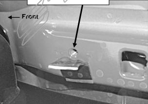
(Fig 3) 2011-12 threaded hole-Nut Plate not required
