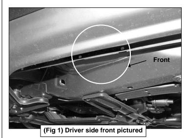
To determine the correct mounting location, locate the three pairs of (2) factory holes in the pinch weld
