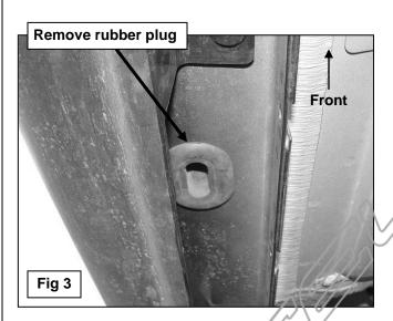
Insert Bolt Plates then rotate clockwise until it stops for proper installation
