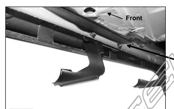
Bolt Mounting Bracket to outside of pinch weld with: (2) 6mm x 25mm Hex Bolts
