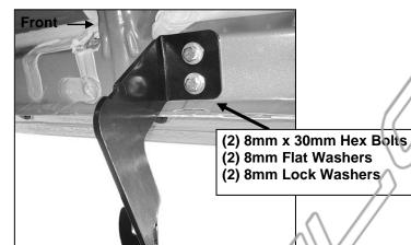
(Fig 3) Driver side center mounting location pictured
