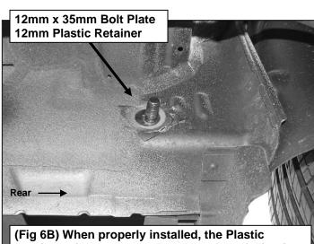
(Fig 6B) When properly installed, the Plastic Retainer will prevent the Bolt Plate from falling into the body panel during installation
