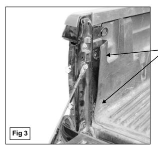
Remove the two hex bolts securing the taillight assembly to the vehicle.
