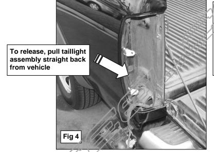
Firmly hold the taillight assembly in both hands and pull straight back from the vehicle to release the taillight assembly from the securing pins.
