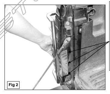
When properly aligned, the gap between the Taillight Guard and the taillight assembly should be the same at the top and bottom. Check the fit all of the way around the Taillight Guard and once satisfied, mark the three locations to drill. IMPORTANT! Remove the taillight assembly before drilling. Do not drill into the body panel with the plastic taillight assembly in place. Do not substitute screws or damage to the taillight assembly may occur.
