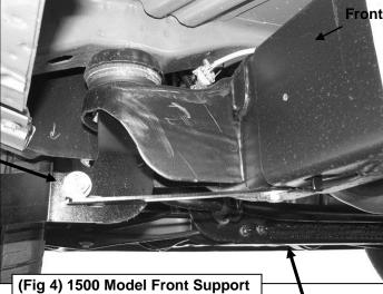
(Fig 4) 1500 Model Front Support Bracket Installation Pictured
