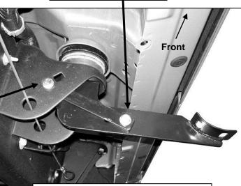
(Fig 7) 25-3500 Model Center Support Bracket Installation Pictured.
