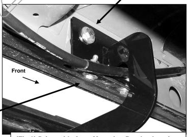
(Fig 2) Driver side-front Mounting Bracket location
