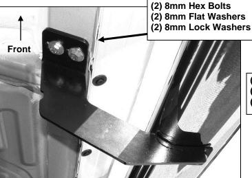
(Fig 3) Driver side center mounting location pictured
