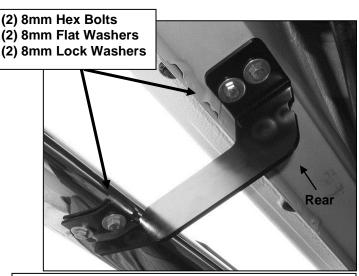
(Fig 4) Driver side rear mounting location pictured
