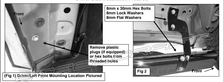
There are four sets of threaded holes in the side panel. Starting from the front of the vehicle, use the first, second, and fourth set of holes.
