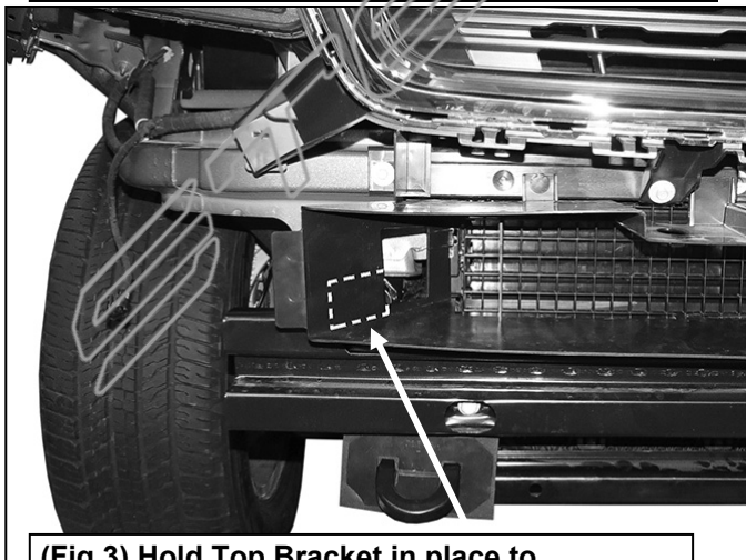
(Fig 3) Hold Top Bracket in place to determine area to cut from air deflector (dashed lines for instruction purposes only)
