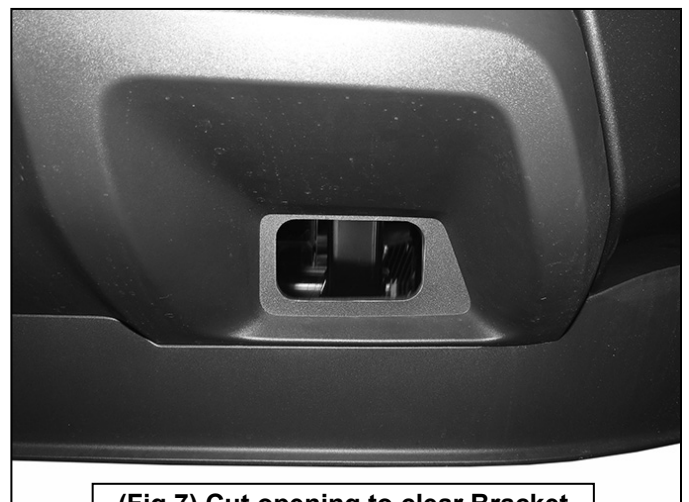
(Fig 7) Cut opening to clear Bracket
