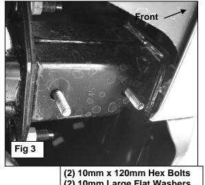
Front **Driver side Frame Bracket** Fig 4A
