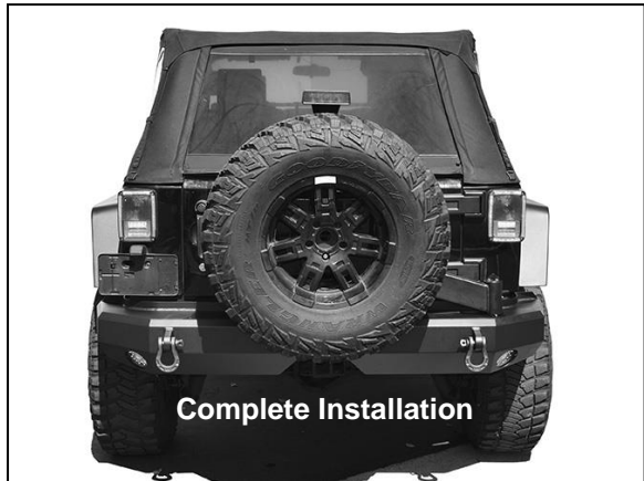
(Fig 21) Attach Top Bracket to Base Bracket. Adjust height to clear spare tire. Plug in light and attach factory 3rd brake light assembly to Bracket
