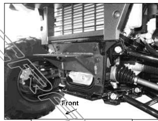
(Fig 4) Winch Mount installed
