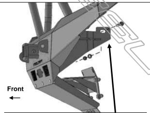
(Fig 8) Reuse factory bolts to attach top mount on back of Bumper to sides of frame
