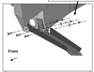
(Fig 7) Attach Bumper to front of Skid Plate
